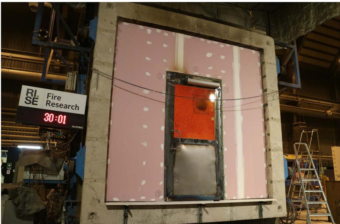
*The test specimen after 30 minutes.*
