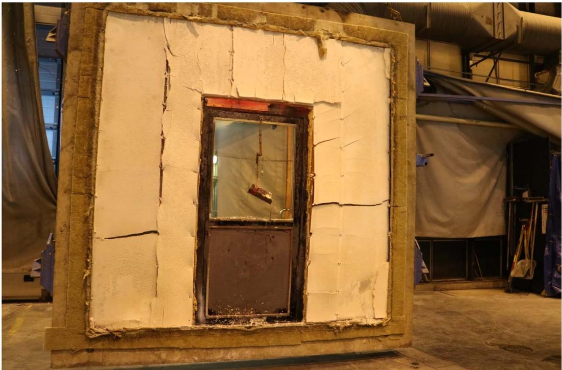
*The test specimen on the fire exposed side after the test.*
