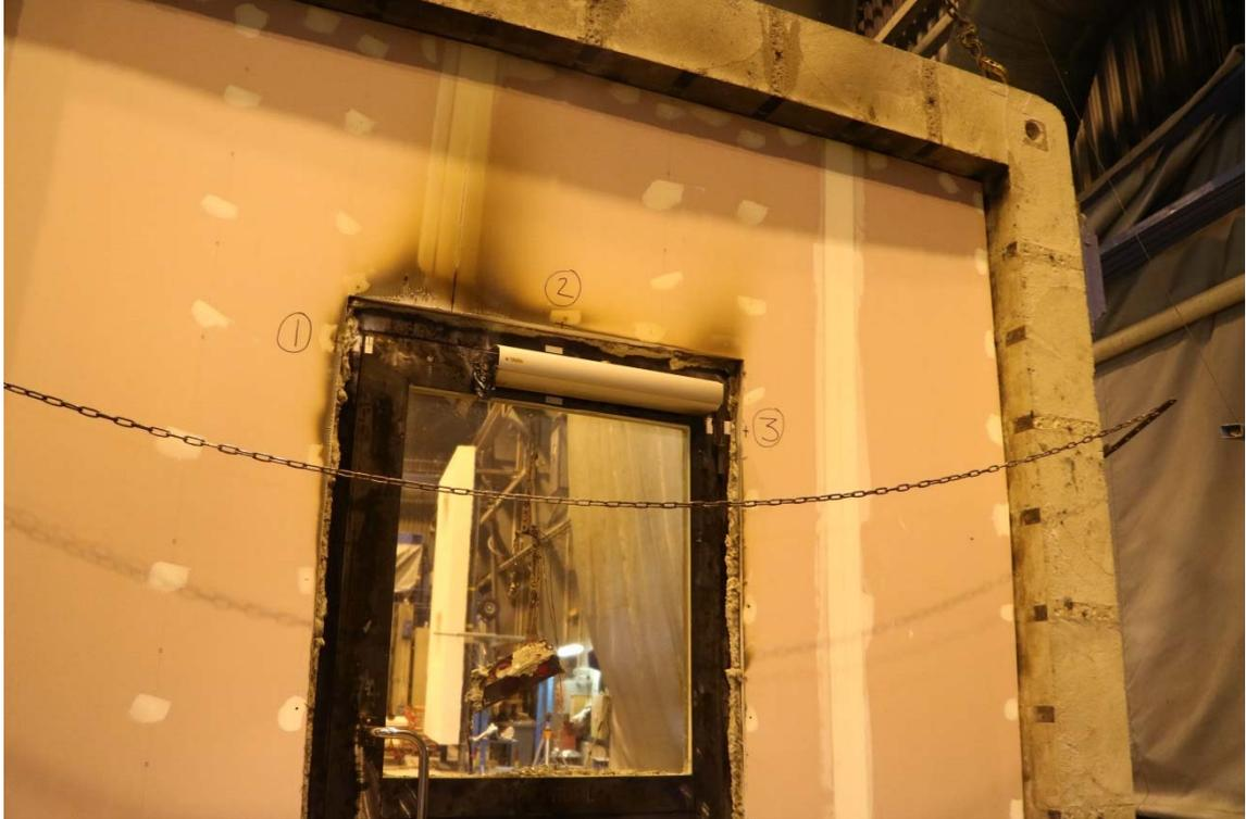
*A close up of the swing door operator on the non-fire exposed side after the test.*
