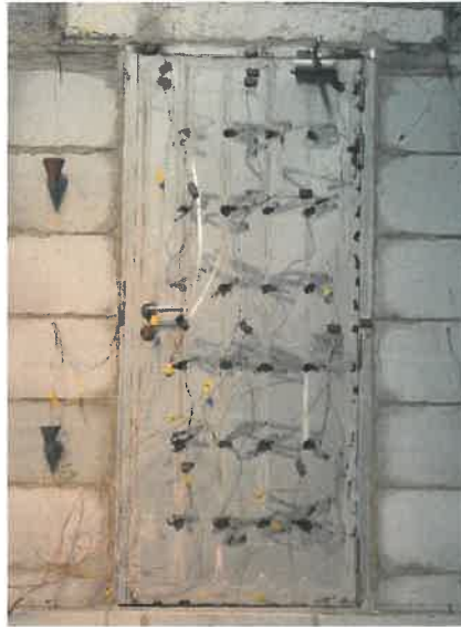
Fig. 5 Unexposed Side after 90 Minutes
