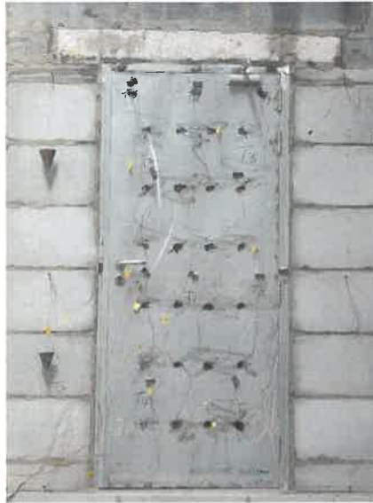
Fig. 3 Unexposed Side after 30 Minutes
