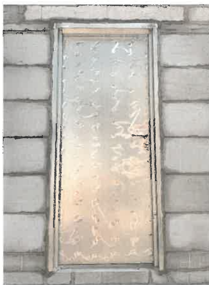
Fig. 1 Exposed Side Prior to the Fire Test
