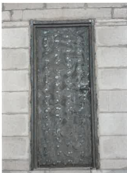
Fig. 8 Exposed Side after 120 Minutes
