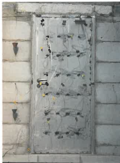
Fig. 4 Unexposed Side after 60 Minutes
